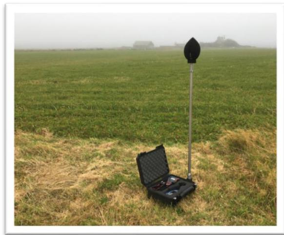
**Figure 3: Noise surveying equipment**
