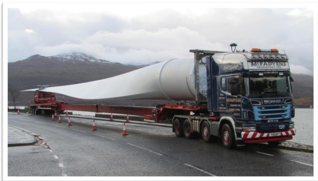
**Figure 4: Example turbine blade in transit**
